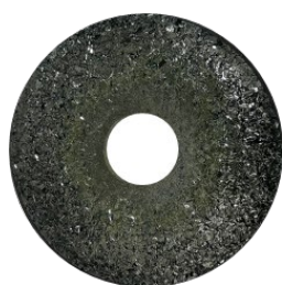
(a) Focus Ring graphite structure
