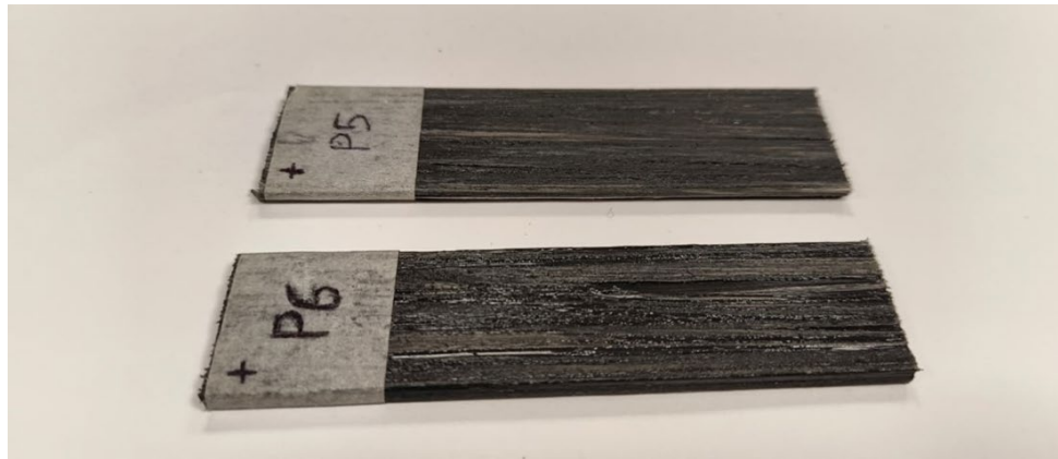
Fig. 4. Pultruded composite (P5 – T200 v120; P6 – T200 v180)
