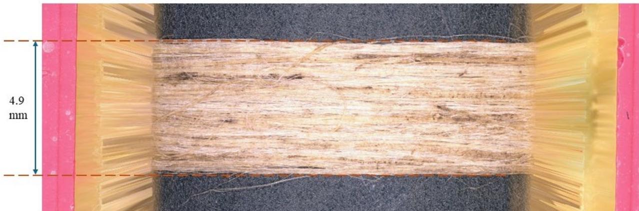
Fig. 2. Compaction device under microscope
