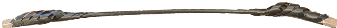
Fig.3. Upon removal from the mandrel, some preforms undergo significant axial expansion and a reduction in their inner diameter
