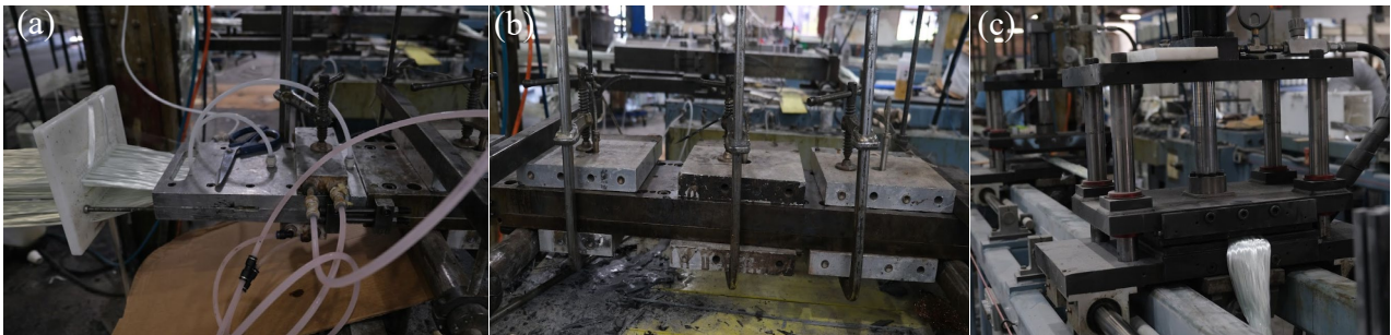
Fig. 1. Schematic of the PulFlex line pultrusion process: (a) resin impregnation via MVP injection box, (b) three-zone heated forming die, (c) in-line puller.
