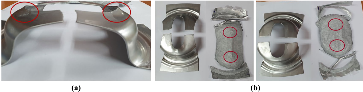
Fig. 9. Deformation of dummy sheets and specimen from uniaxial tension to plane strain.
