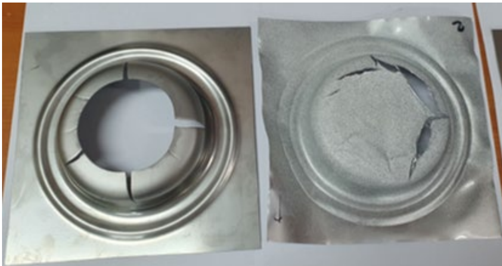
Fig. 10. Failure of dummy sheet and specimen in equi-biaxial loading.
