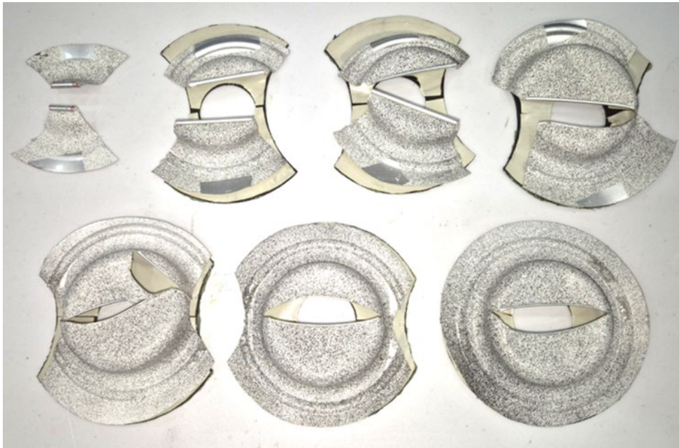
Fig. 13. Fractured specimens after forming limit test results with EPDM dummy sheets.
