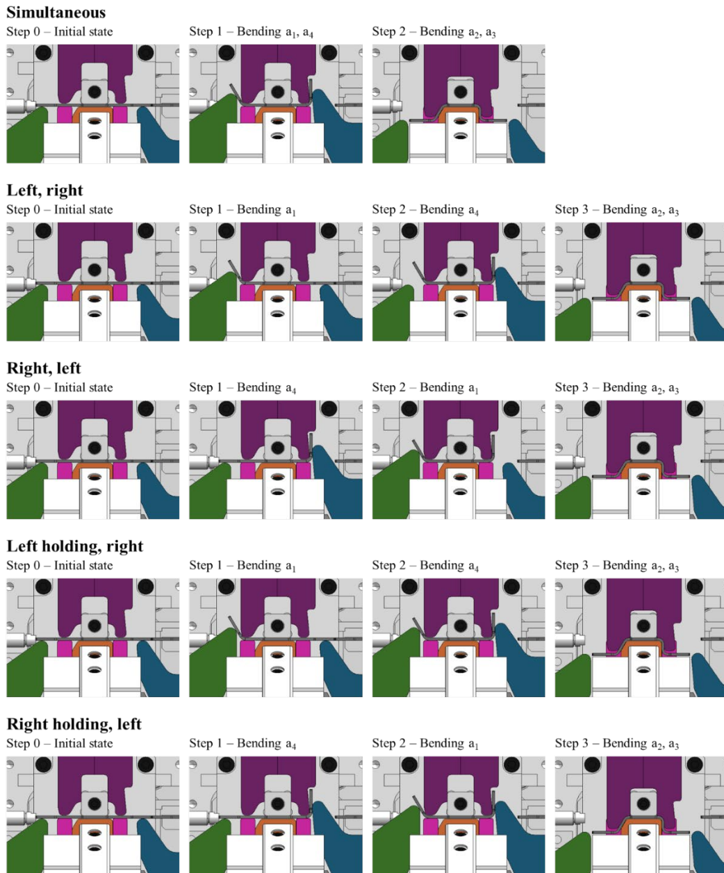
Fig. 5. Positions of the bending punches for the five different bending sequences.
