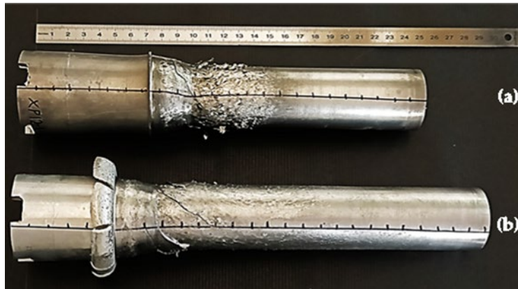
Fig. 4. Deformed parts at the end of CFT experiments on (a) mat-W+3h and (b) mat-O specimens.
