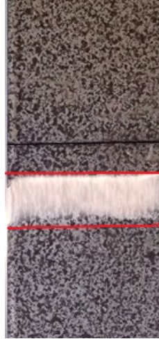
Fig. 6. Short tensile test specimen. Deformation only takes place between the two red bars. The specimen elongation is tracked with a video system on the undeformed gray pattern.
