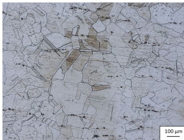
Fig. 3. Initial microstructure of Inconel 718
