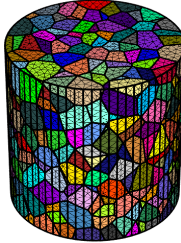
Fig. 1. RVE created by Neper to be used in CPFEM simulation.
