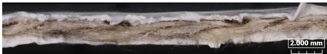
Fig. 7. Failure surface from a penetration test on a deformed laminate
