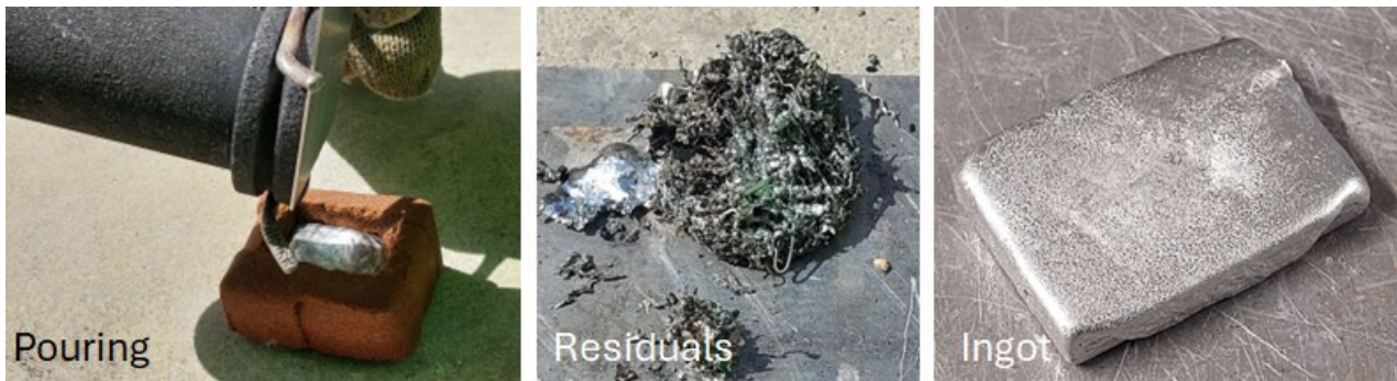
Fig. 4. Manufacturing of an ingot with the recovered soldering alloy.
