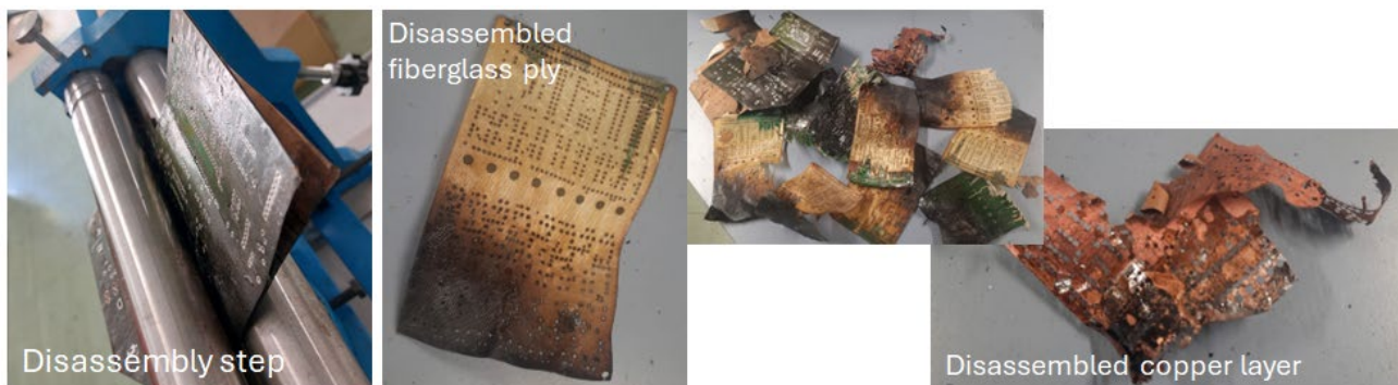
Fig. 5. Copper extraction from waste PCBs by thermo-mechanical disassembly.
