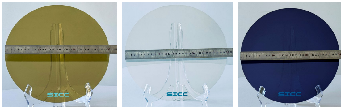
Fig. 5. Images of fabricated 12 inch n-type SiC substrate, 12 inch high-purity SiC substrate and 12 inch p-type SiC substrate.
